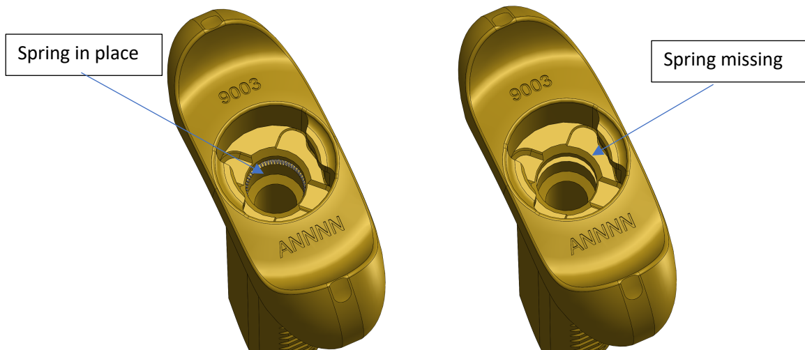
5) Figure 9: Handle Assembly illustrating spring placement.
